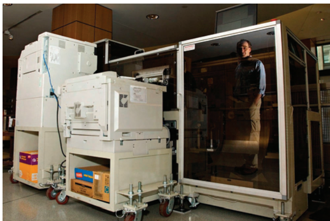
On Demand Books, started by a former Random House editorial director, is beta testing its Espresso Book Machine. The device can print black-and-white text for a 300-page paperback, with a four-color cover, and bind it all together in three minutes at a cost of $3.
